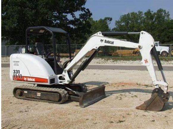
Figure 11: Mini excavator for access road works
