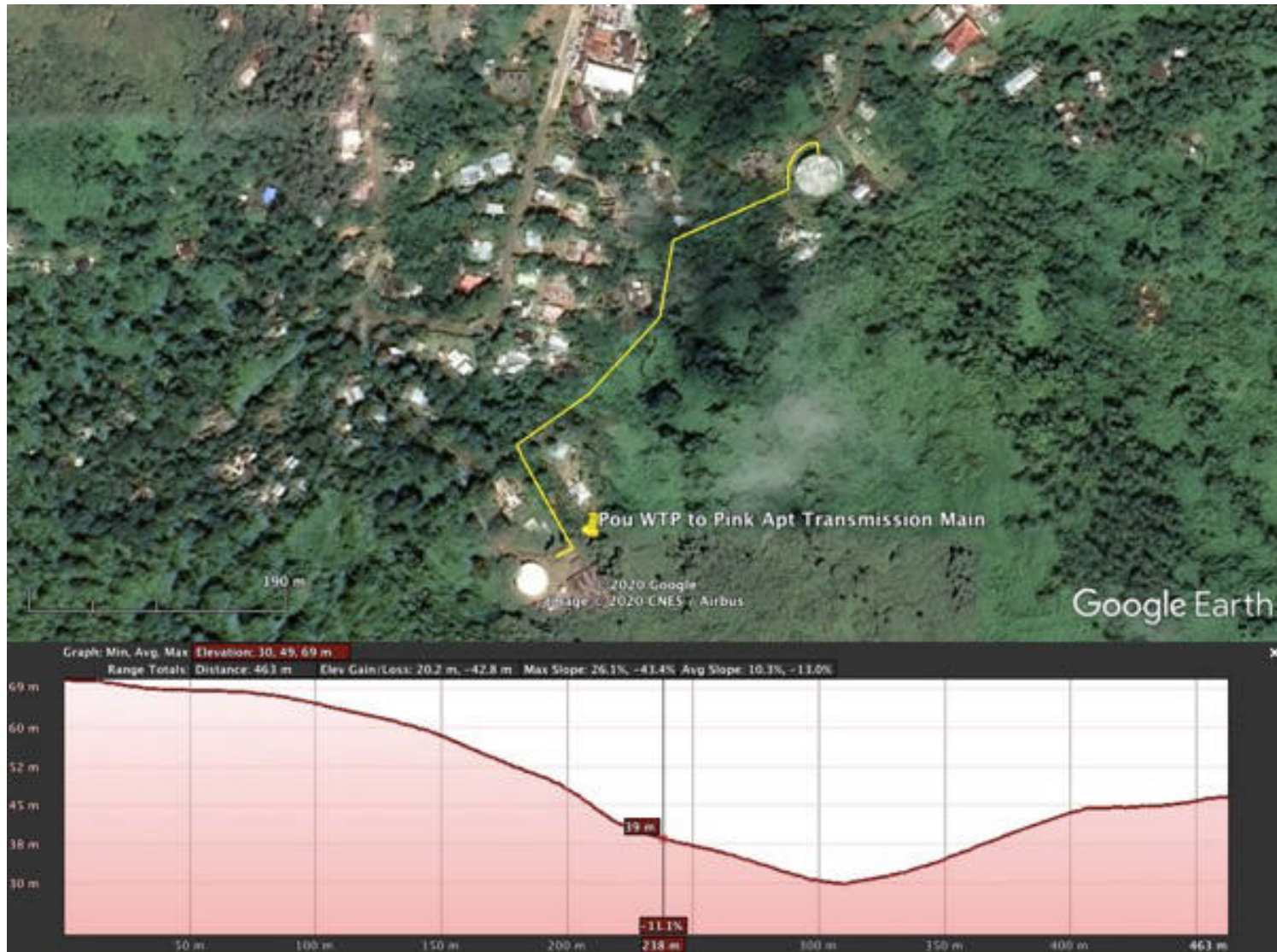
Figure 12: Construction of a Transmission Line Directly Linking the Pou WTP Storage Reservoir to the Pink Apartment Storage Reservoir
