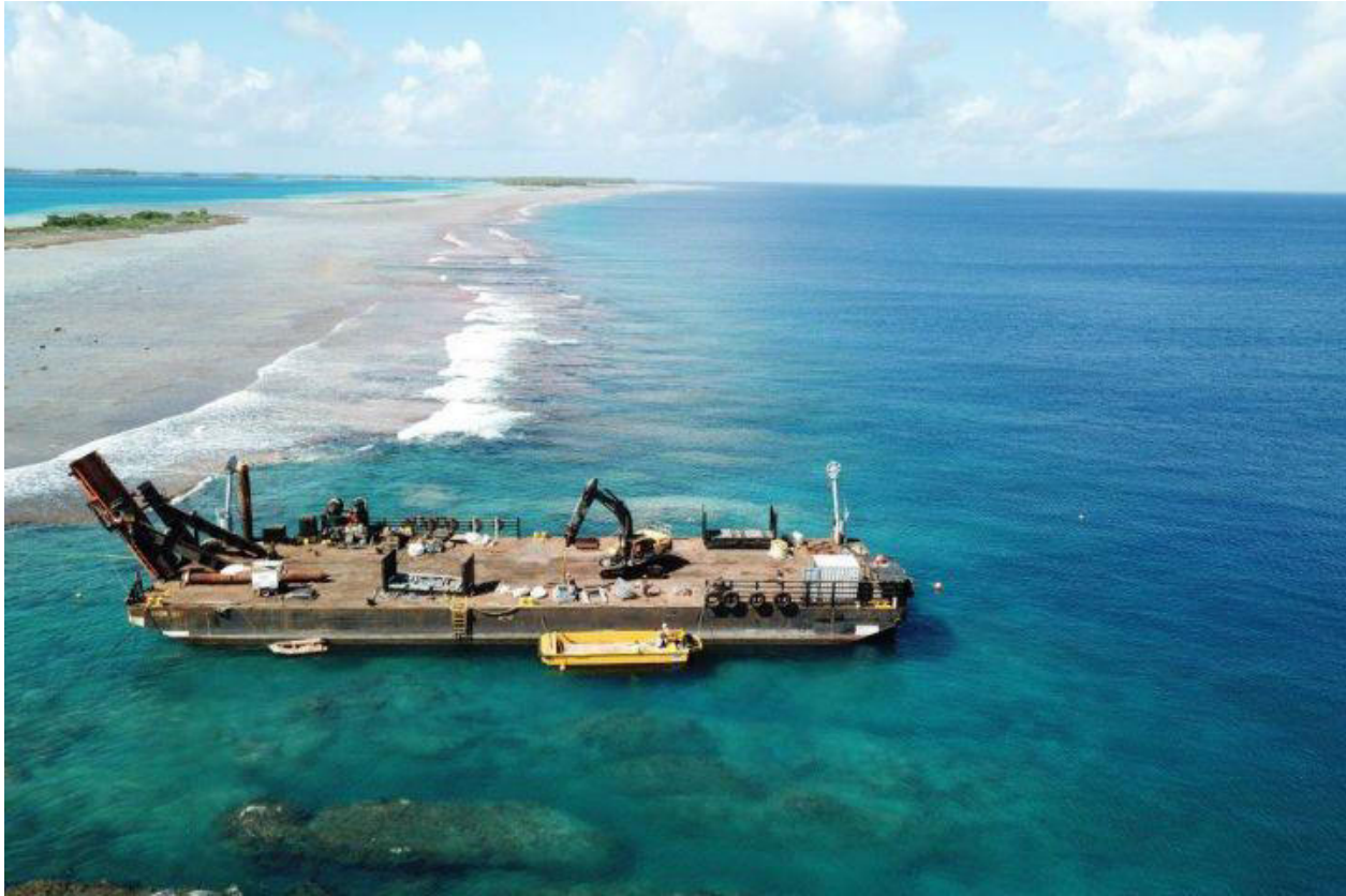
Plate 5.4: Suggested dredge plant – large spudded barge (the Orion) with 80t long reach excavator
