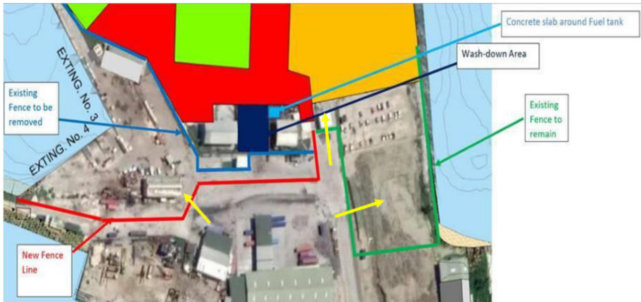
Figure 3.21: Proposed bunding arrangements for the construction phase (access in yellow)
