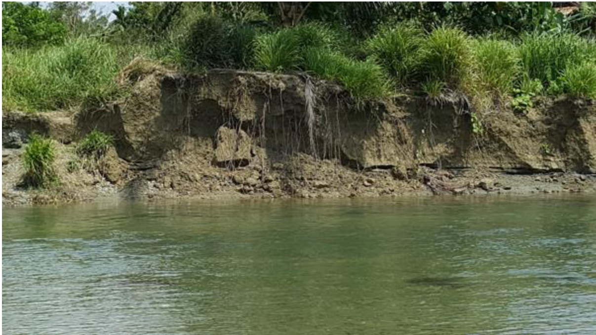
Figure 23: Moderately Erodible Siltstones on Banks of Mongga River near site
